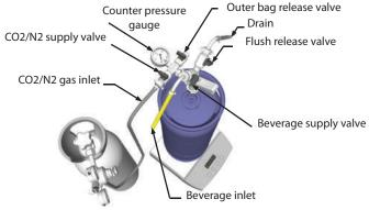
Fill the supply hose: Open, then close the beverage supply valve to fill the supply hose, then clean the head with ethanol.
